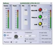
Adjust the incoming microphone gain via the XLR or headset connection. The Glensound Referee compressor is automatic and prevents clipping, but a further multi stage compressor can be added to balance the audio signal. A meter will show real time input level.
